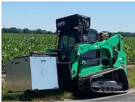
Figure 3: "LightSpeed" electro-fluids impulsive source.
