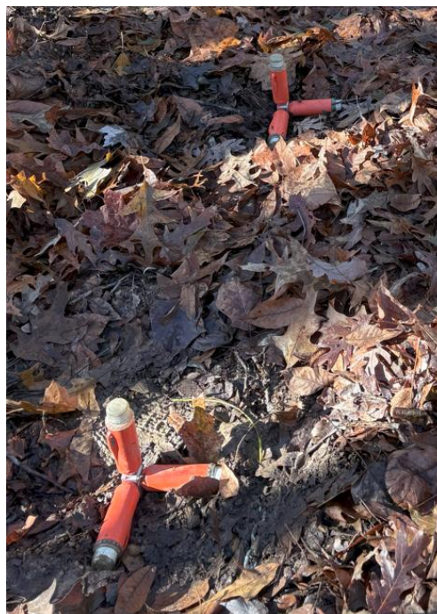
Figure 2. Field deployment of three single component Stryde nodes configured as a 3C receiver. The photo shows two (2) separate 3C receiver stations at the 1m receiver interval used on the project.
