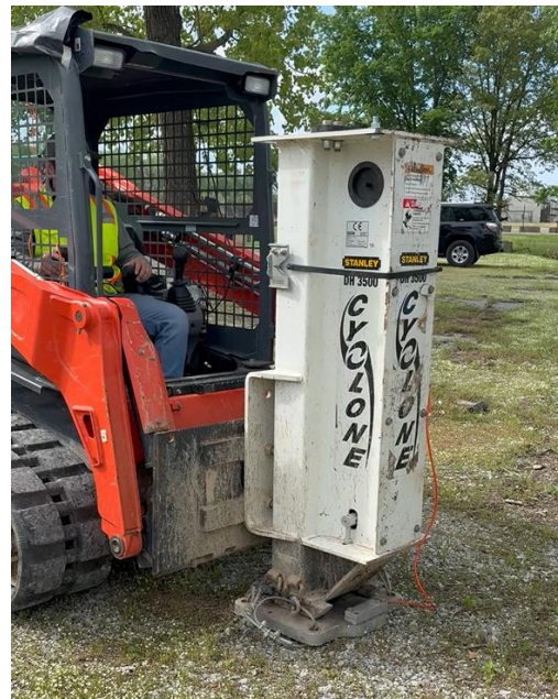
Figure 4: Compressional weight drop source.
