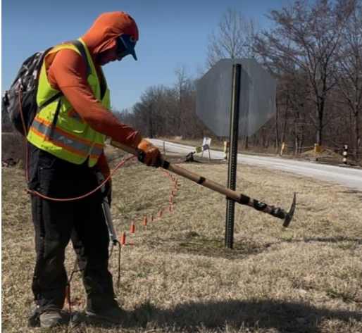
Figure 5: Shear energy I-beam and hammer source.
