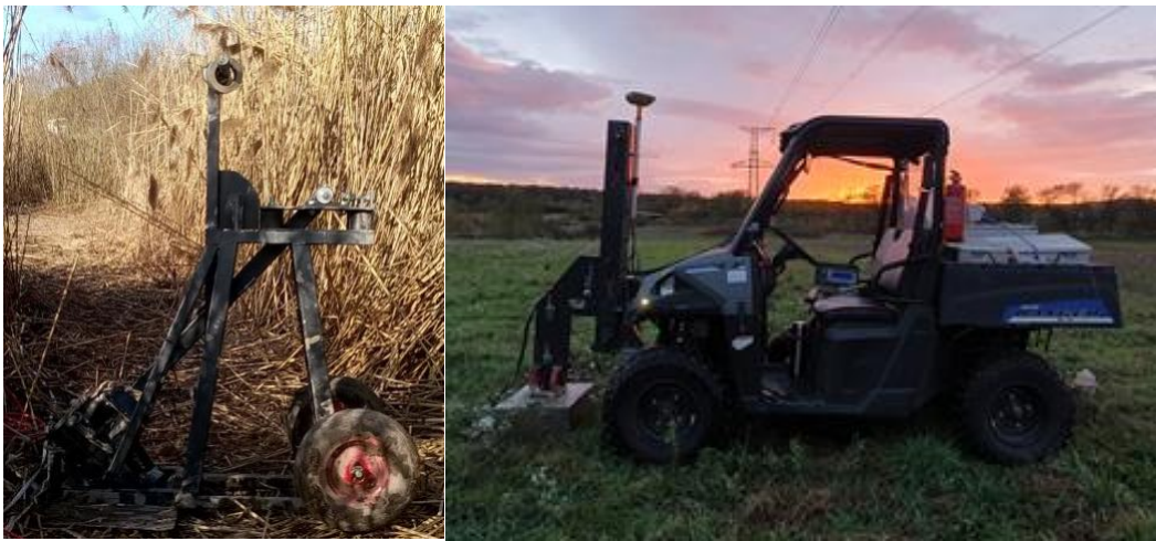
Figure 3 S-wave seismic sources used for the 3D seismic survey were combination of hammer (left image) and Lightning eVibe manufactured by Seismic Mechatronics (right image)
