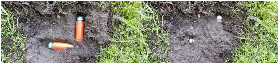
Figure 4 2C S-wave recording with STRYDE system placed in two horizontal directions in the ground
