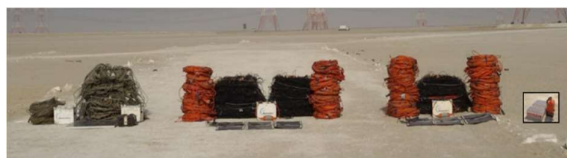
Figure 2 – 1 km of acquisition equipment used for the 2D line layout, from left to right: single sensor cabled system, array cabled system 12 geophones, array cabled system 6 geophones, the new nimble node system at same scale (inset)
