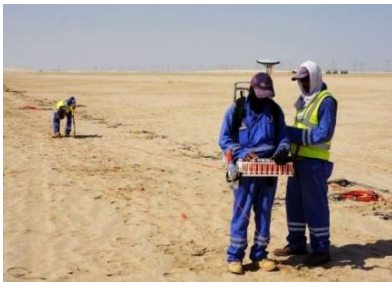
Figure 3 - a 3-person crew deploying the new nimble node.
