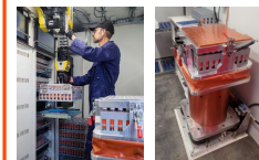
Figure 4: mechanized loading of modular, high-capacity, charge/download racks (left) and automated node tester (right) enables scalable camp operations
