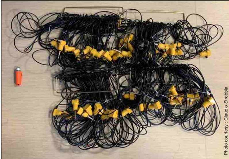
Figure 1- Single sensor STRYDE node size compared to cabled geophones
