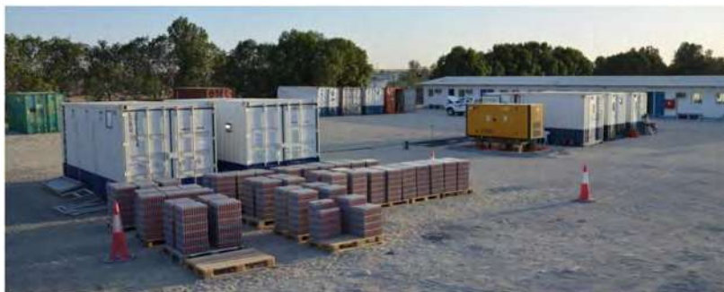
Figure 1—The field camp where the field trial operation was conducted. 20-foot Containers from left to right hold respectively: the charging and harvesting unit, the cleaning unit, the data storage unit, the recording truck unit and the workshop unit. In front on the pallets we can see approximately 35,000 nodes
