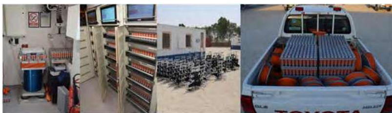
Figure 2—from left to right: the calibration table, the charging and downloading racks, the deployment and retrieval backpacks, a pick-up loaded with 1600 nodes and 20×600m string reels.
